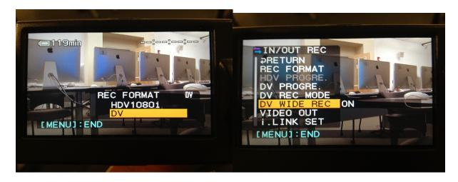
1. Set your camera to DV (standard definition) before plugging your camera in. This is an Edition limitation and can be resolved by purchasing Wirecast Studio and the HDV plugin (or using DOM's equipment).
