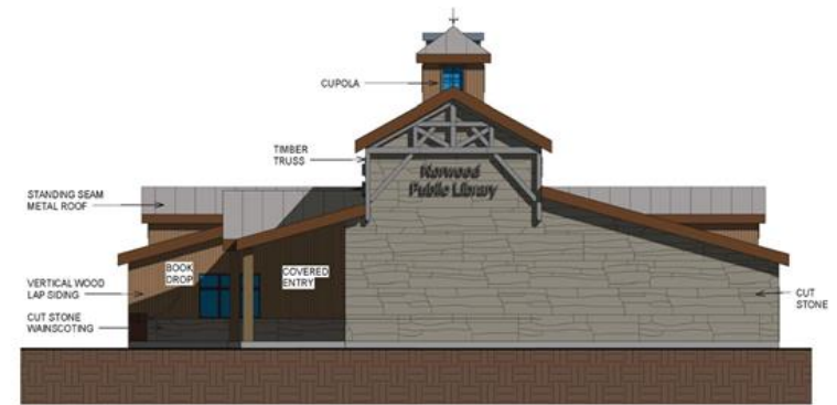
② NORTH EXTERIOR ELEVATION 3/32" = 1'-0"
