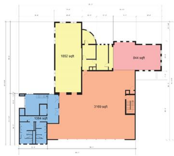
Building Additions Plan - Main Level
