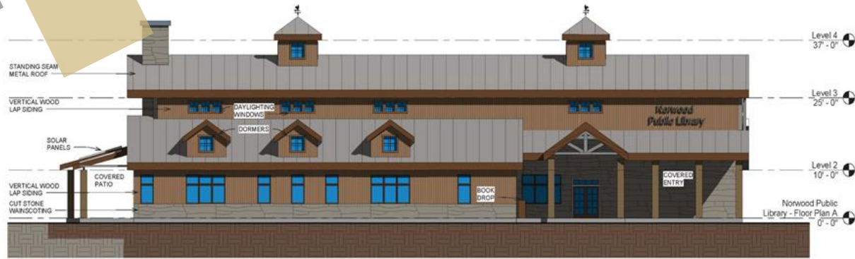
① EAST EXTERIOR ELEVATION 3/32" = 1'-0"
